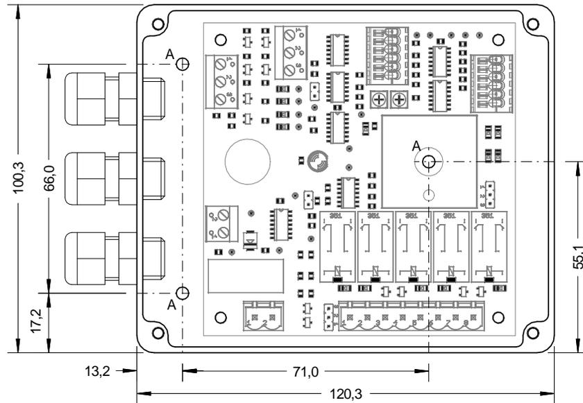
A = 3x Bohrung Ø 3,6mm
